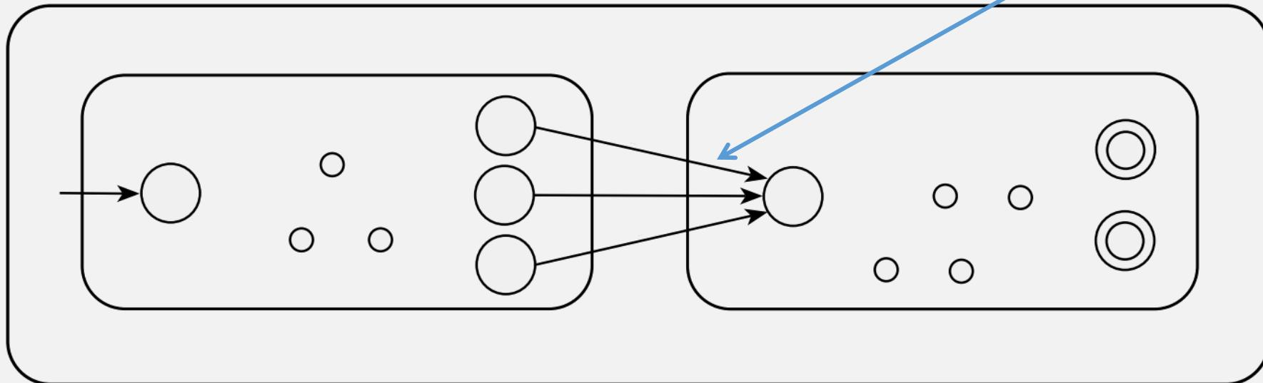
**Concatenation:**  $A \circ B = \{xy \mid x \in A \text{ and } y \in B\}$
